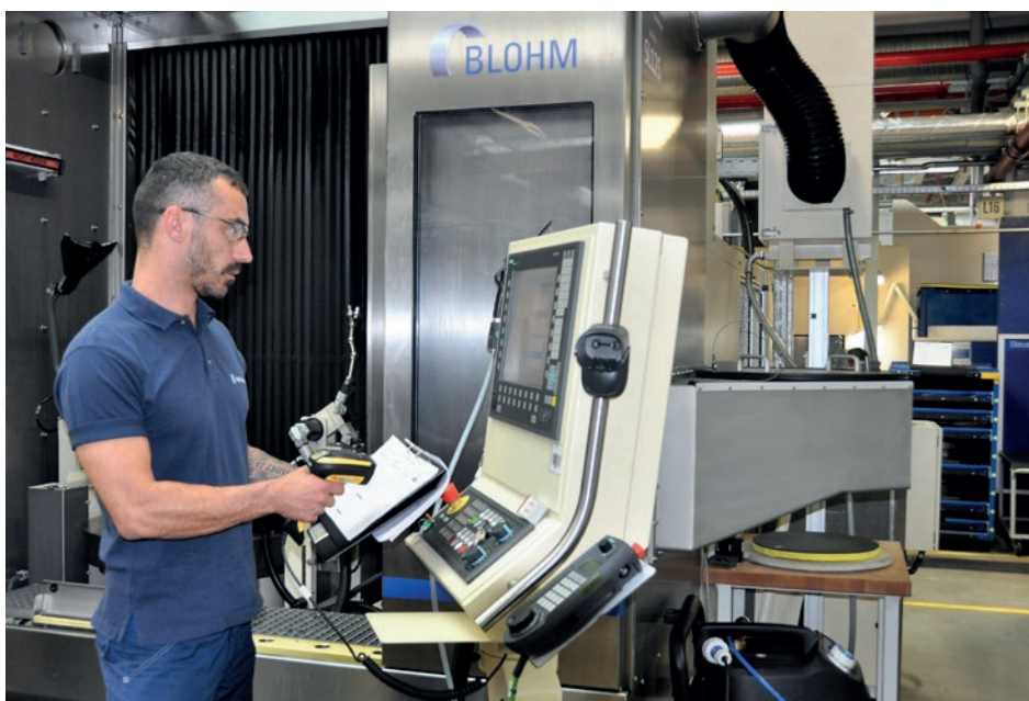
For Tim Riegelhof the hand scanner makes things much easier. The data have scarcely been read in, before the software automatically sets the workpiece-specific NC program.
